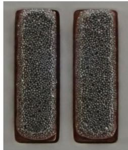
**Figure 8. An example of a good stencil printing on PCB.**
