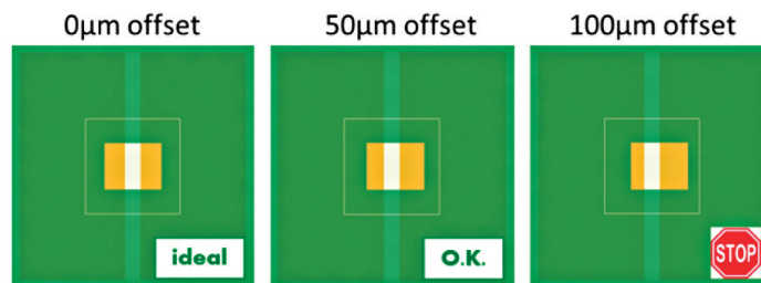
Figure 16. Solder mask registration offset to copper trace
