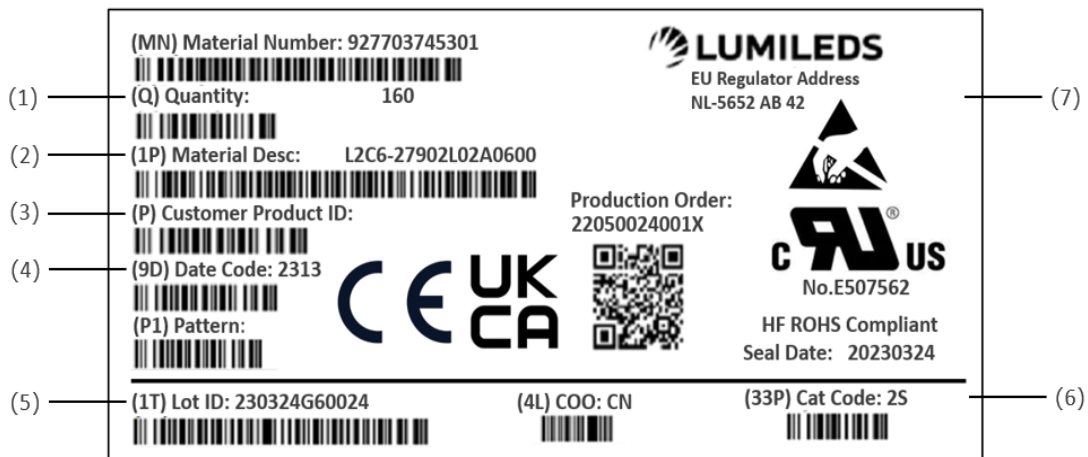
Figure 11. Example of inner box label and tray label for LUXEON CS CoB.
