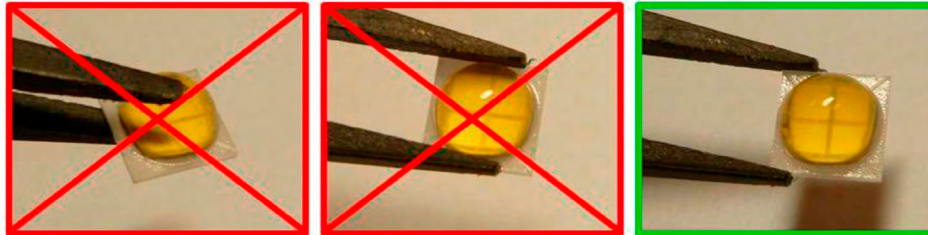
Figure 4a. Illustration of incorrect handling (left & middle) and correct handling (right) of a representative domed LED package similar to LUXEON SunPlus HPE.
