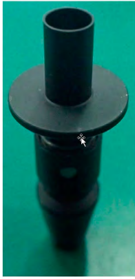
Figure 12. Nozzle design for Samsung SM421 (part number: SAM-0712/16, drawing number: 13994B from Ching Yi Technology Pte. Ltd., ( http://www.chingyi.com.sg ). All dimensions are in millimeters.
