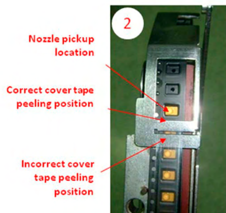
Figure 15. Three representative feeder designs. Feeder 1 does not require any modification. Feeder 2 requires the cover tape peeling position to be shifted. Feeder 3 requires the shutter to be removed before the cover tape peeling position can be adjusted.
