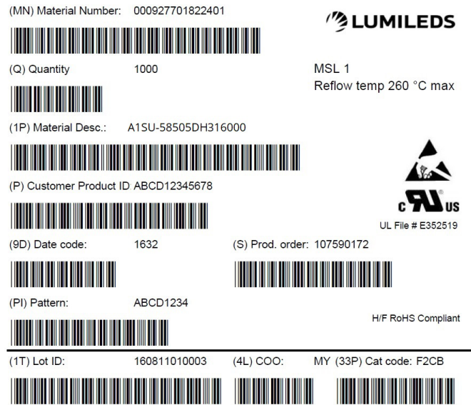
Figure 13. Example of a product label for LUXEON Altilon TopContact.
