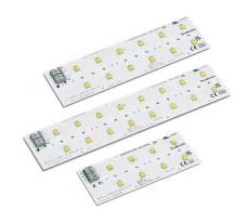
LUXEON XR-5050 Round products are LED modules optimized for lighting applications requiring high efficacy LED arrays mounted on a rigid and thermally conductive substrate. These versatile building blocks feature 8, 12, and 16 LUXEON 5050 LEDs on a MCPCB substrate, are designed for ease of system integration, faster time to market, and use with industry standard optics. LUXEON XR-5050 Round is a complete solution combined with standard third-party optics and heatsink.
