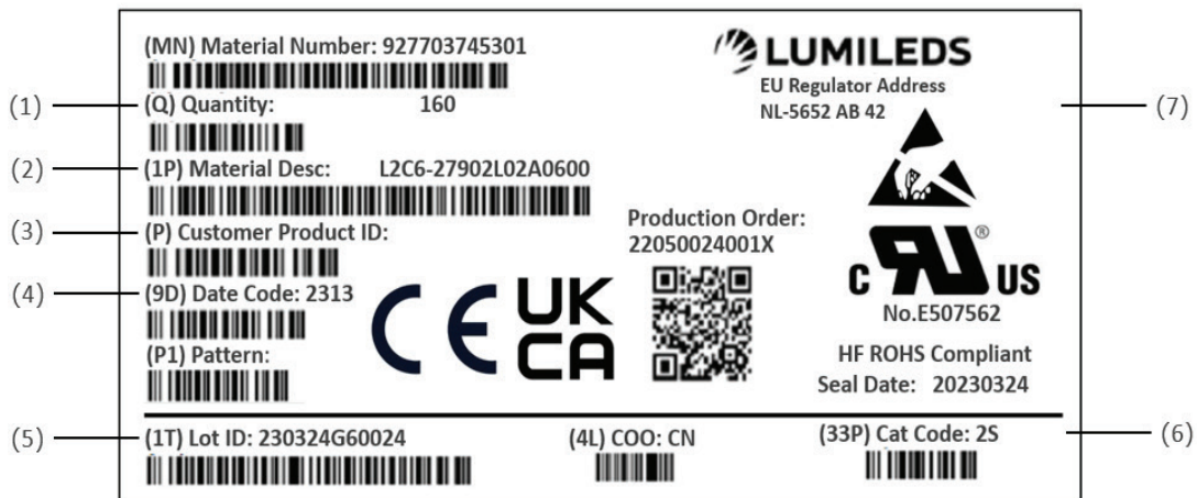
Figure 10. Example of inner box label and tray label for LUXEON CS CoB
