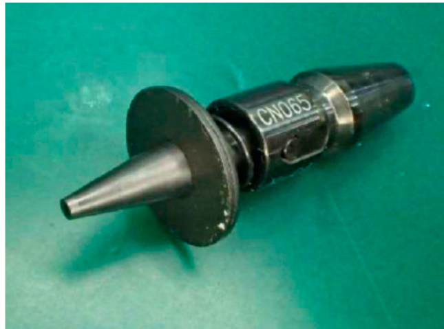
Figure 20. Standard off-the-shelf nozzle “CN065” (inner diameter 0.65 mm, outer diameter 1.2 mm) with Zirconia tip for Samsung SM421 machine.
