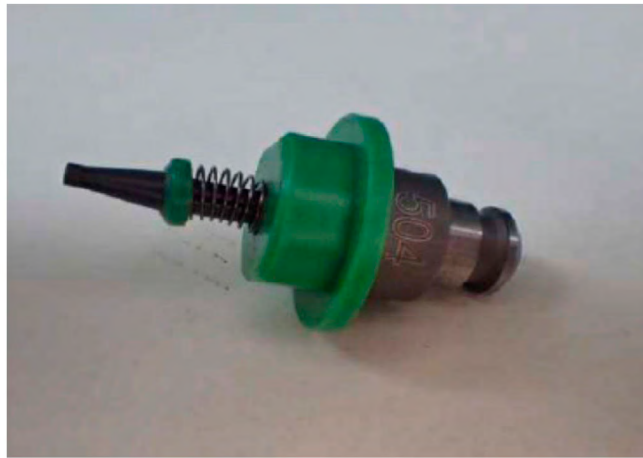
Figure 21. Standard off-the-shelf nozzle "504" (inner diameter 1.0mm, outer diameter 1.5mm) with Zirconia tip for Juki KE-2080L machine.
