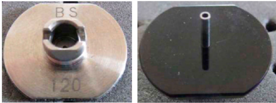
Figure 22. Standard off-the-shelf nozzle “120” (inner diameter 0.9 mm, outer diameter 1.3 mm) with metal tip for Panasonic CM402 machine.
