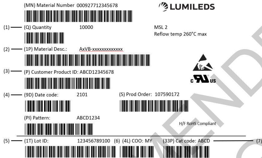
Figure 12. Example of a moisture barrier bag and reel label for LUXEON Versat 2020 140
