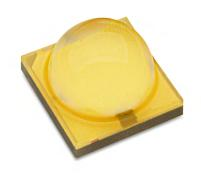
LUXEON V is a Chip Scale Package (CSP) based high power emitter designed to deliver maximum flux in a compact 4.0mm x 4.0mm footprint. LUXEON V offers a unique combination of high efficacy at high drive current with extremely low thermal resistance and optimized radiation pattern to support next generation fixture designs. Building on the strengths of Lumileds Patterned Sapphire Substrate (PSS) CSP technology, LUXEON V offers the highest drive current capability in its class.
