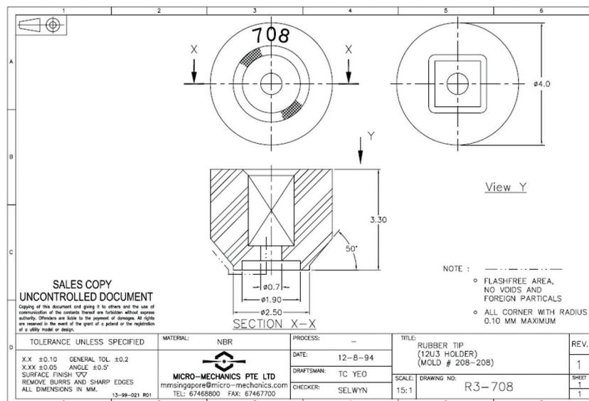
Figure 17. Standard nozzle for LUXEON Altilon SMD 1x3 and 1x2 LED array.
