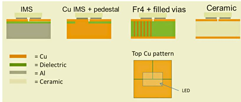
Figure 10. Layer stacks and top side pattern.
