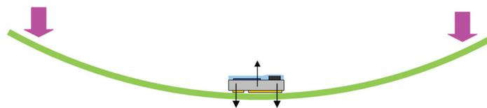
Figure 24. Board warpage after reflow.
