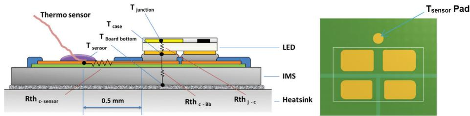
Figure 12. Temperature probing by thermo sensor (schematically).
