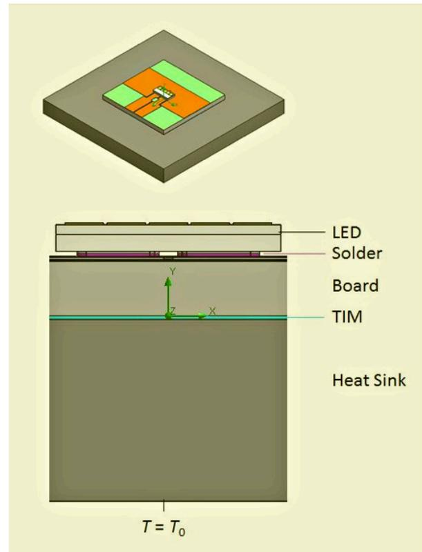
Figure 9. Model geometry of LUXEON Altilon SMD.
