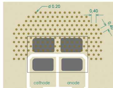
Figure 11. FR4 design with filled and capped via.
