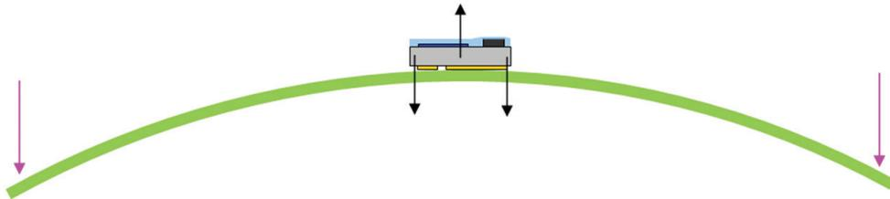
Figure 22. Forces acting onto package when board is bent.
