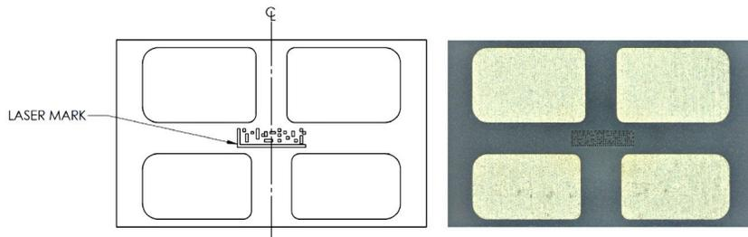
Figure 4. Example of a dot matrix code on bottom side of LUXEON Altilon SMD.
