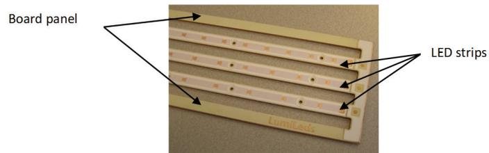
Figure 23. PCB panel consisting of several strips of LEDs.
