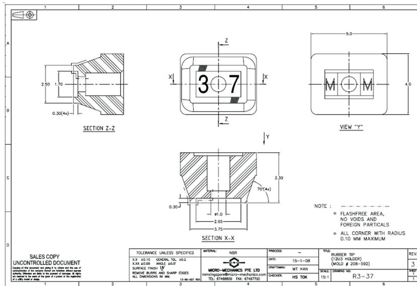
Figure 16. Standard nozzle for LUXEON Altilon SMD 1x5 and 1x4 LED array.
