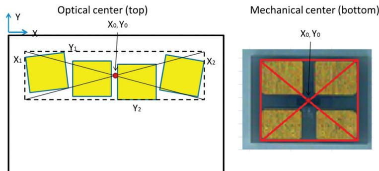
Figure 19. Definition of optical and mechanical center for LUXEON Altilon SMD.
