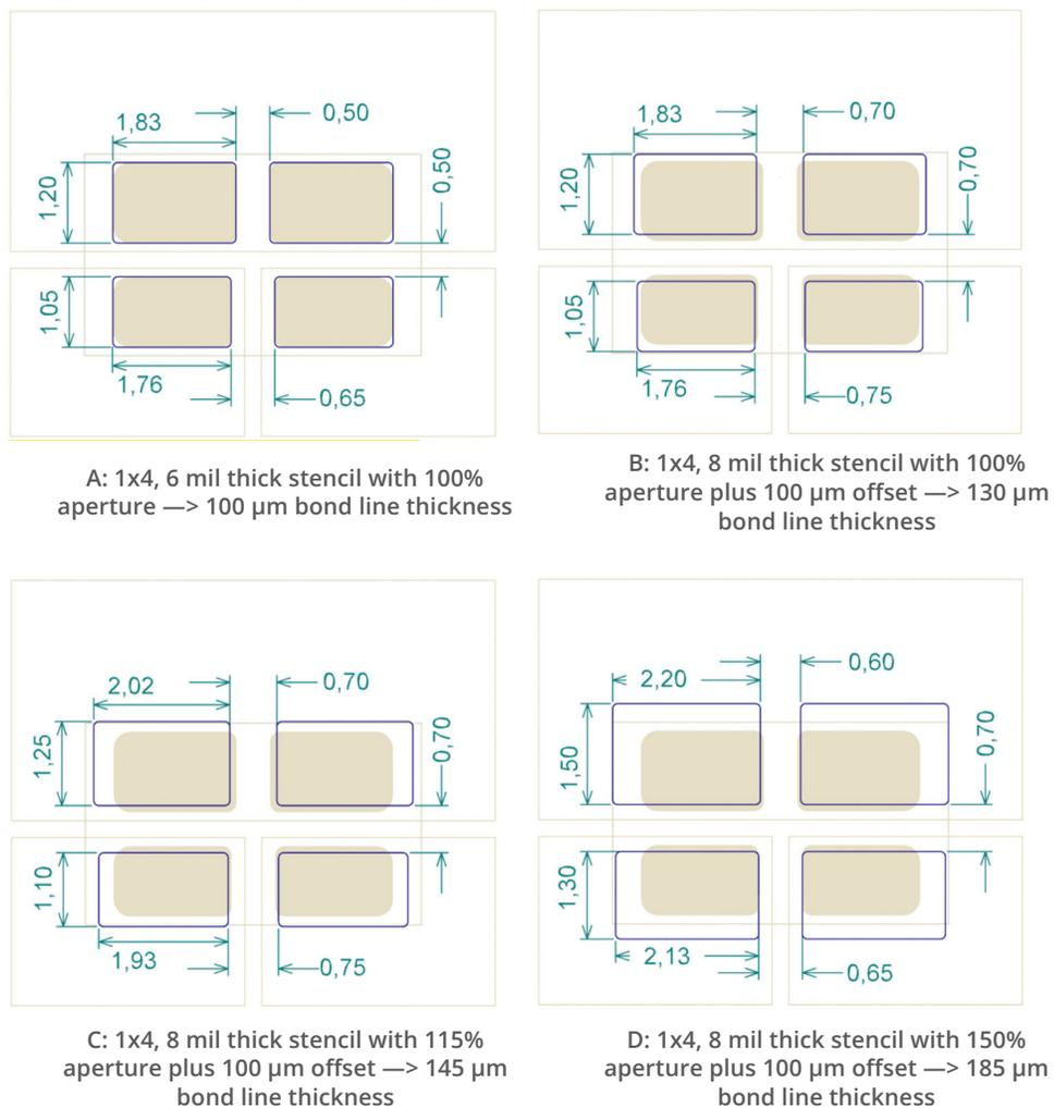
Figure 13. Stencil aperture designs for LUXEON Altilon SMD.
