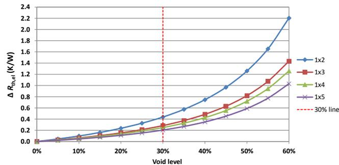
Figure 20. Impact of voids in the solder joint on the thermal resistance. The thermal resistance values are based on electrical input power.
