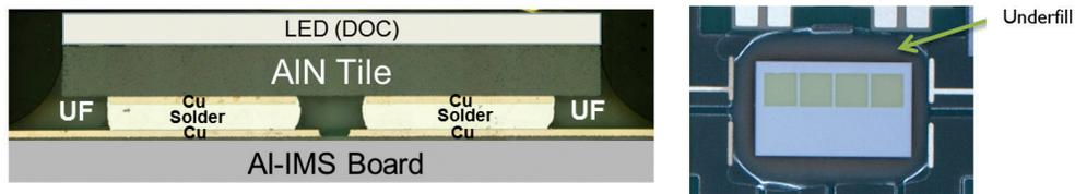
Figure 21. Cross section LED with Underfill.
