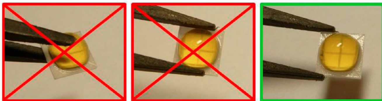
Figure 3a. Illustration of incorrect handling (left & middle) and correct handling (right) of a representative domed LED package similar to LUXEON HL2X-V.
