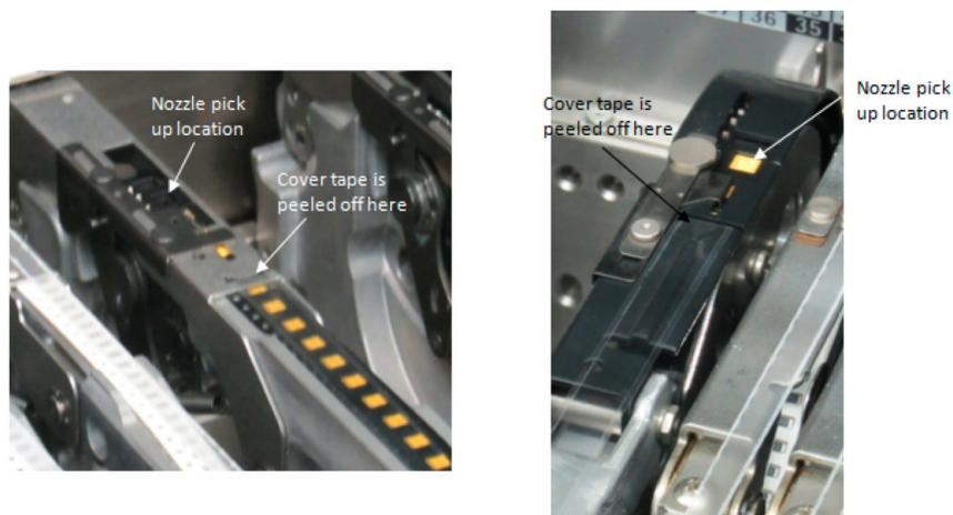
Figure 14. Examples of Samsung SM421 (left) and Juki KE-2080L (right) pick and place feeders used to pick and place LUXEON domed packages.
