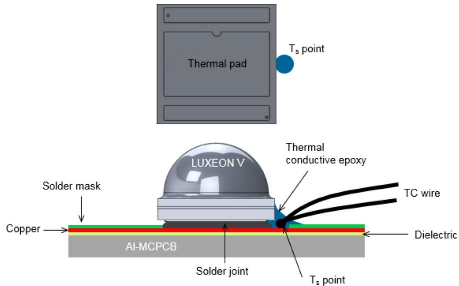
Figure 8. Drawings showing the recommended location of the  $T_s$  point (top).
