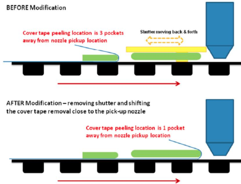
Figure 15. Illustration of the general principle behind the feeder modification where, in some cases, there may be a need for the LED emitter to be picked up immediately after the cover tape is peeled off.
