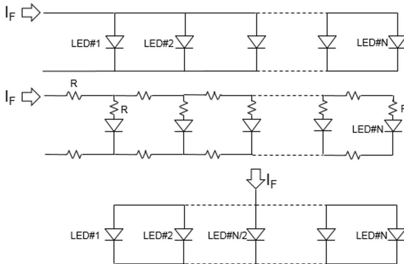
Figure 6. Effect of trace resistance and routing pattern on LED light output performance as described.
