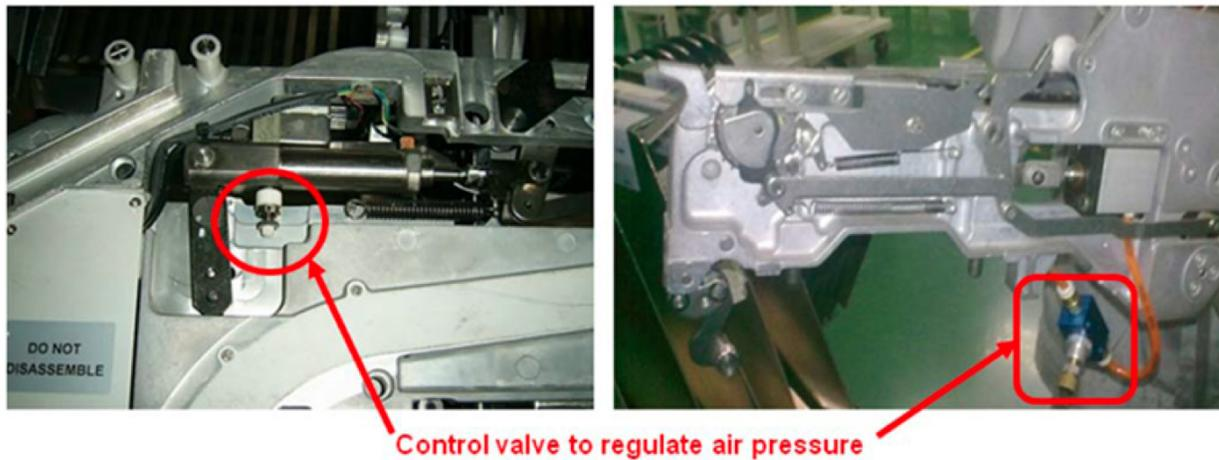
Figure 17. Pneumatic feeder with integrated air pressure control valve (left) and modification made to the pneumatic feeder by installing air pressure control valve (right).
