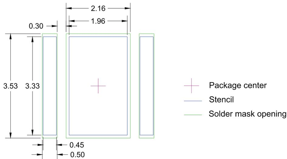
Figure 4. Recommended footprint layout for LUXEON V. All dimensions are in millimeters.
