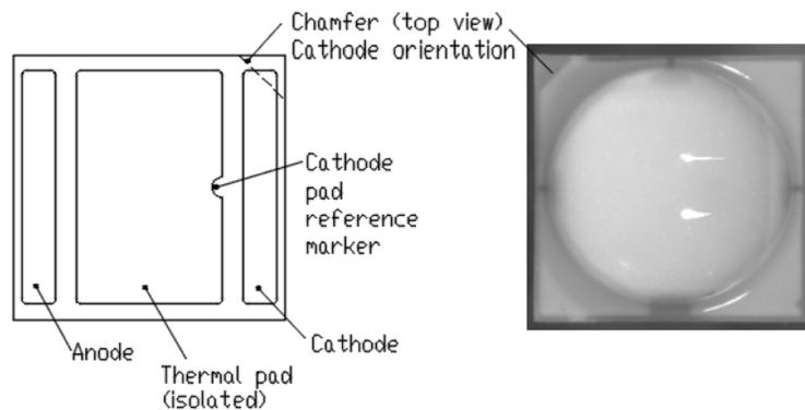
Figure 1. Bottom view (left) and top view (right) of the LUXEON V LED.
