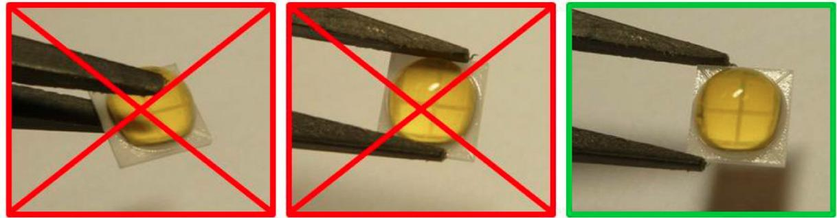
Figure 3. Incorrect handling (left & middle) and correct handling (right) of a domed LED package similar to LUXEON V.
