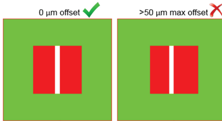
Figure 9. A maximum of 50µm mis-registration between solder mask (green) and copper pattern (red) is preferred.
