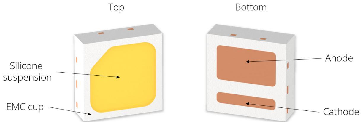
Figure 1b. Top view (left) and bottom view (right) of the LUXEON Versat 2020 Cool White / PC Amber
