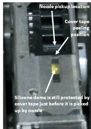
Figure 21: Example of a modified feeder which protects the silicone dome prior to pickup.
