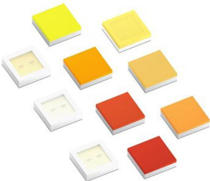
Designed with space and energy efficiency in mind, LUXEON HL1Z Colors deliver deep hues from a small package, with minimal power consumption. This is enabled by CSP (Chip Scale Package) technology with an LED size of only 1.4mm x 1.4mm. This product line is both suited for applications with individual emitters as well as multicolor clusters.
