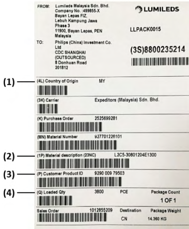
Figure 14. Example of outer box label for LUXEON CoB Core Range PW.
