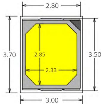
Figure 5. LUXEON 2835 emitter in a tape pocket with inner dimensions of 3.0mm x 3.7mm. A suitable starting point is to choose a nozzle size where the x or y dimensions or the diameter (if round nozzle) is larger than the yellow region and able to rest on the outer white plastic housing. Dimensions in mm.
