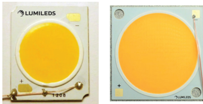
Figure 5. The recommended temperature measurement point T_s is located on the circular gold pad at lower right hand corner of LUXEON CoB 1208 emitter on the PCB (left). Note: LUXEON CoB 1321 and CoB 1825 emitters have a shared location for T_s and Cathode pad (right). T_c must be placed where it will not interfere with the electrical connection
