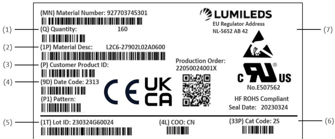
Figure 11. Example of inner box label and tray label for LUXEON CS CoB with CrispColor Technology.
