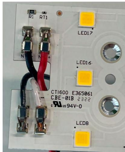
Figure 5. Illustration on inserting wire on a representative Lumileds LED module.
