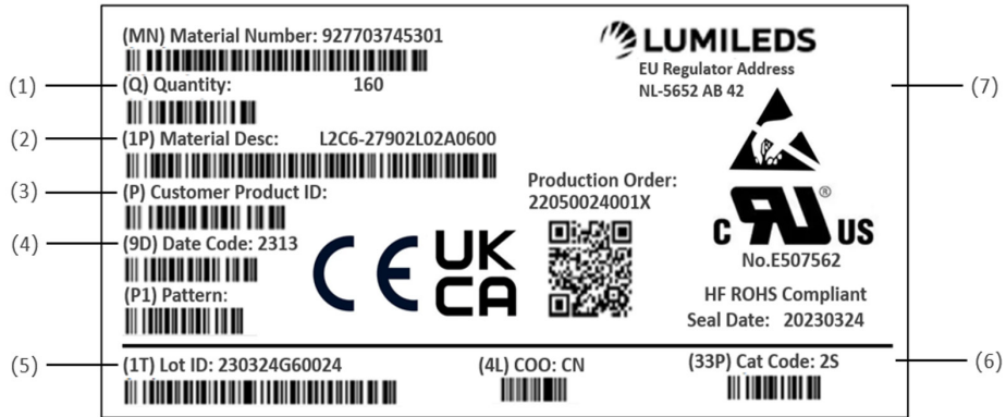
Figure 11. Example of inner box label and tray label for LUXEON CS CoB with CrispWhite Technology
