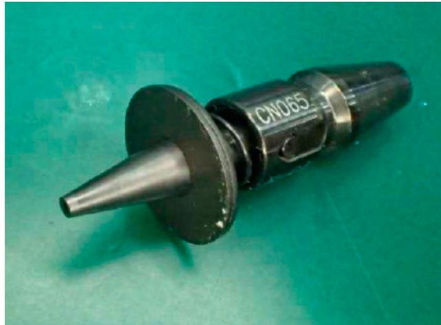
Figure 19. Standard off-the-shelf nozzle “CN065” (inner diameter 0.65mm, outer diameter 1.2mm) with Zirconia tip for Samsung SM421 machine.
