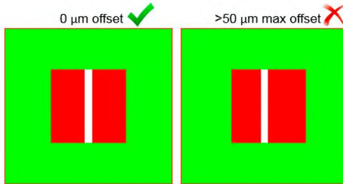
Figure 9. A maximum of 50 $\mu$ m mis-registration between solder mask (green) and copper pattern (red) is preferred.
