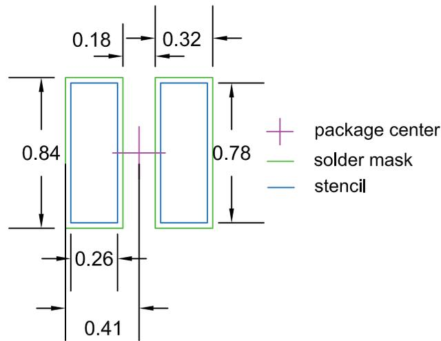
Figure 5. Recommended bottom pad drawing of LUXEON HL1Z. All dimensions in mm.
