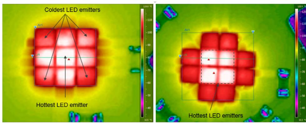
Figure 23. Thermal imaging camera results for LED clusters (150 $\mu$ m spacing) with close packing on Al-MCPCB (1oz copper, 3W/(m.K) 100 $\mu$ m dielectric).
