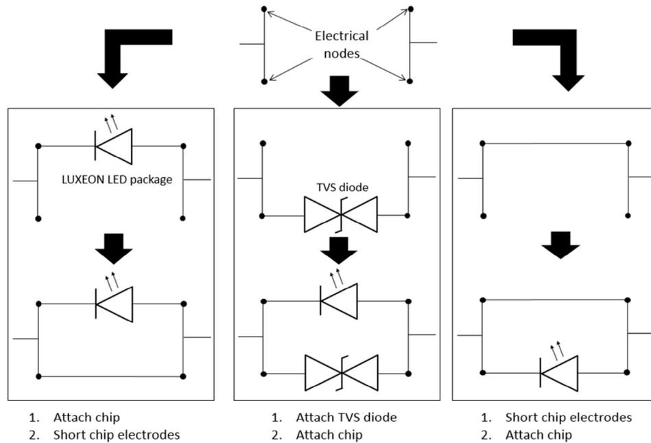
Figure 21. Electrical schematics showing three different methods of ESD protection. The middle picture provides permanent ESD protection while the left and right pictures are temporary solutions. It is important that device shorting should only be done if you know that static build up is not present by practicing safe ESD handling at all times.
