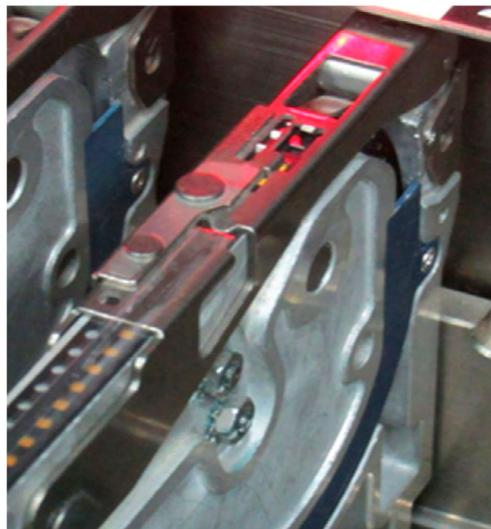
Figure 15. Samsung SM421 feeder.
