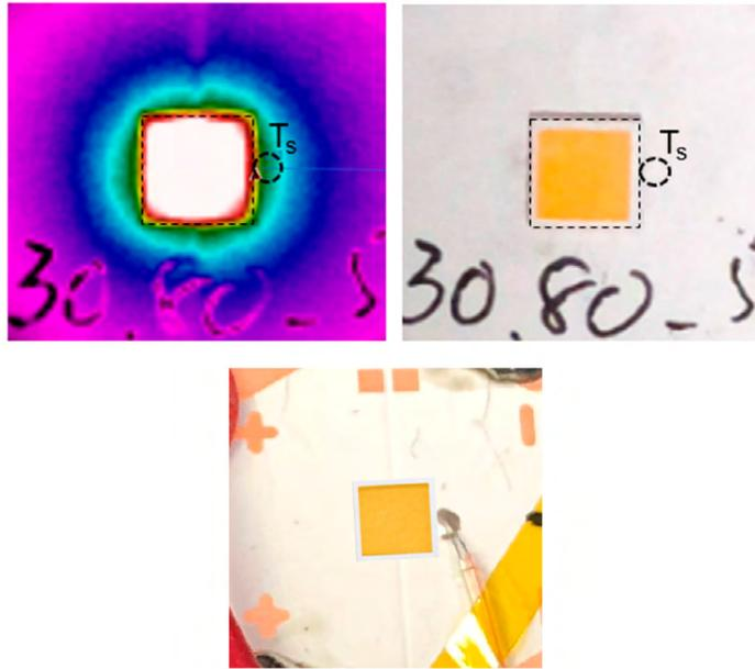
Figure 22. Shown here is a representative LED package. The  $T_s$  location should be placed close to the package as shown. The  $R\theta_{j-s}$  is characterized based on this placement position. The further away the  $T_s$  point is, the calculated junction temperature will then be under-stated.
