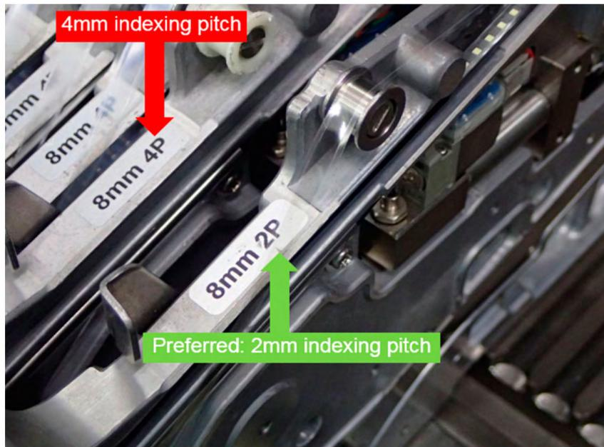
Figure 16. An example of Samsung SM421 feeder with 2mm and 4mm indexing pitches. Smaller indexing pitch creates smoother feeder motion.
