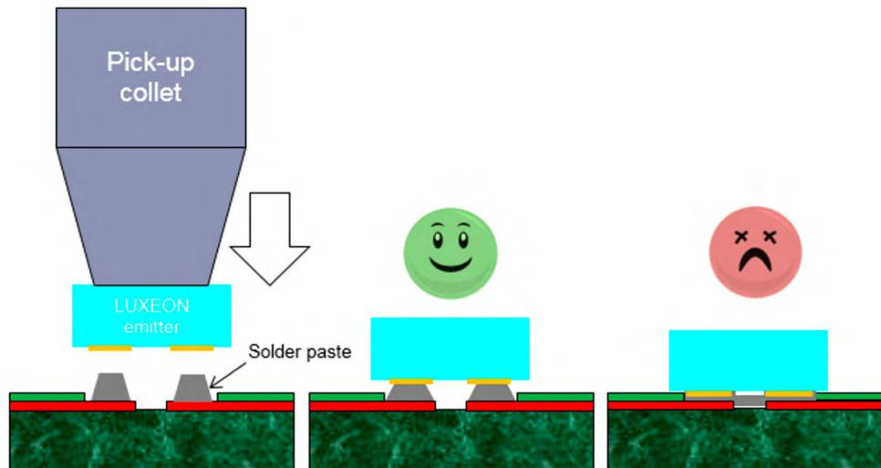
Figure 18. A proper starting point for the mounting z-height of LUXEON HL1Z is  $\frac{1}{3}^{\text{rd}}$  of the stencil thickness with reference to the top of the stencil paste, i.e. the collet should be in an under-travel position. Center picture shows the optimum result for the collet height setting. Right picture shows over-travel position and may result in bridging of the solder paste on adjacent pads prior to reflow, increasing the likelihood of electrical shorts.
