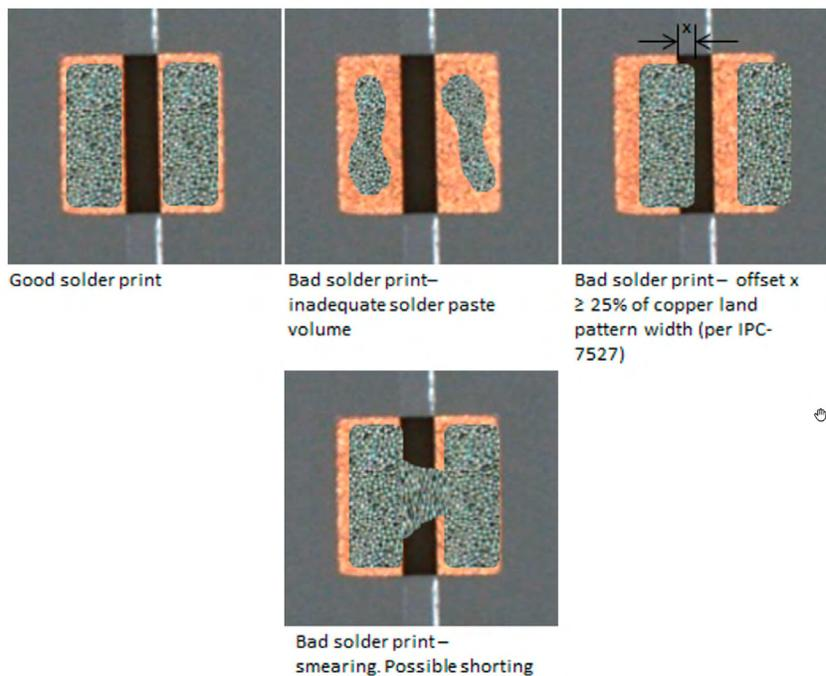
Figure 11. Examples of good and bad solder print.
