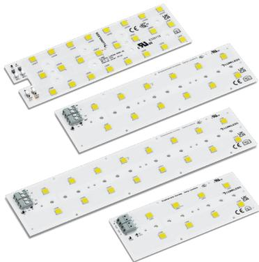
LUXEON XR-5050 HE integrated modules are standard products compatible with off-the-shelf drivers, optics, and heat sinks. These versatile building blocks feature 8, 12, 16 or 24 LUXEON 5050 HE LEDs on a MCPCB substrate for thermal efficiency and mechanical robustness. This approach simplifies system integration and accelerates time-to-market.
