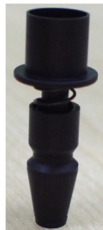
Figure 6. Samsung SM421 nozzle (metal). Dimensions in mm.
