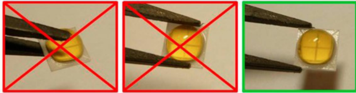
Figure 3a. Illustration of incorrect handling (left & middle) and correct handling (right) of a representative domed LED package similar to LUXEON HL4X.
