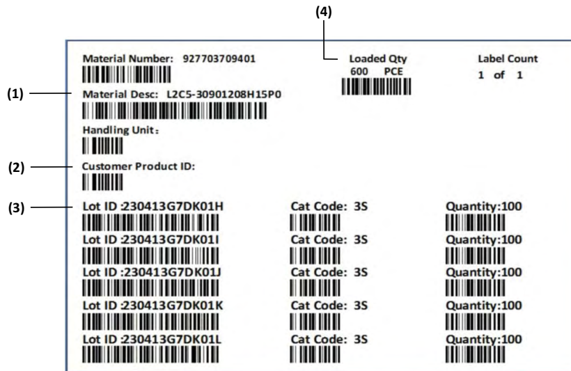
Figure 14. Example of outer box label for LUXEON CoB Core Range High Density Gen 2.
