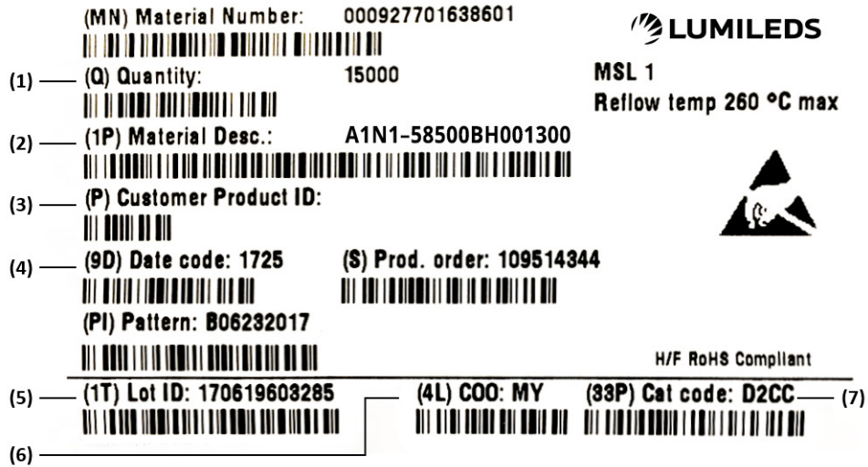
Figure 13. Example of a reel label for LUXEON Neo 0.5mm 2 .
