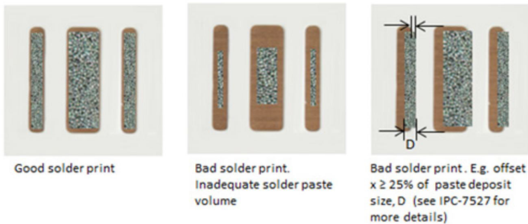
Figure 12. Examples of good and bad solder paste printing on two and three pad emitters. Visual inspection of the quality of the dispensed solder paste is recommended during process setup or during troubleshooting.
