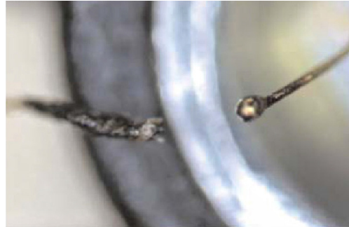
Figure 1. Damage to LED wire bond due to Electrical Overstress (EOS).
