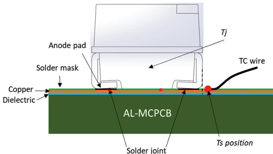
Figure 3. Cross sectional view of LUXEON 3735 Color on Al-MCPCB and the corresponding temperature location. Actual mounting of thermocouple wire closest to the Cathode pad of the LUXEON 3735 Color package on Al-MCPCB.
