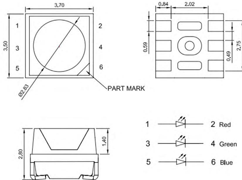
Figure 1. Mechanical Drawing of LUXEON 3735 RGB.
