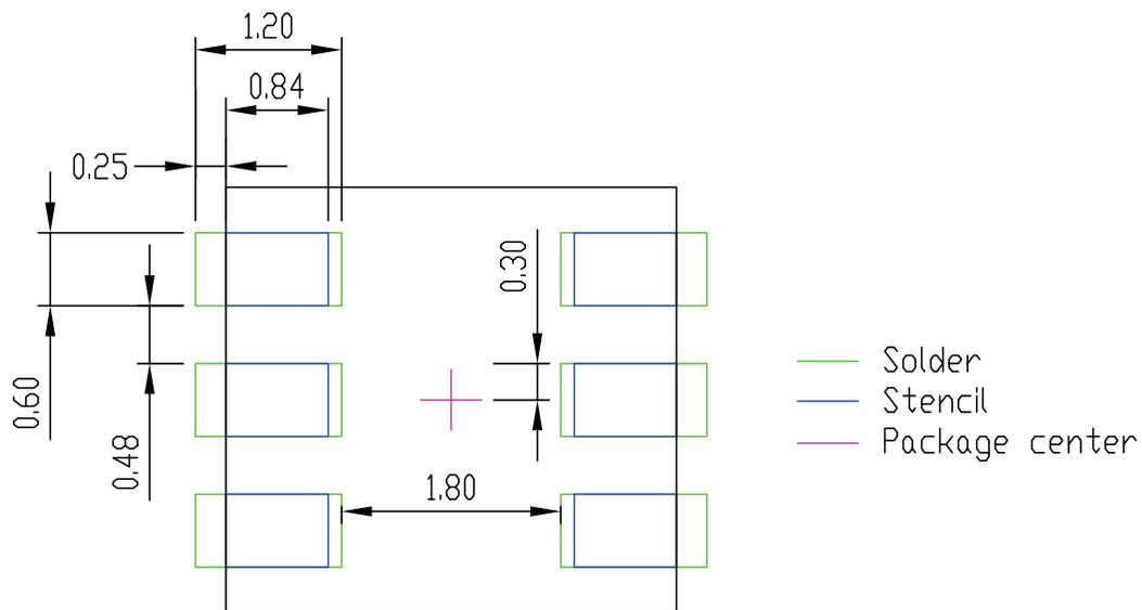
Figure 2. Recommended PCB solder pad layout for LUXEON 3735 RGB.
