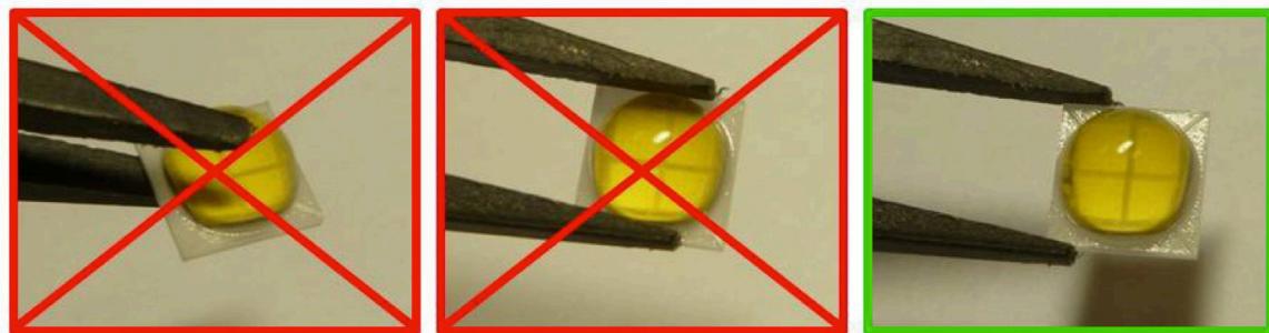
Figure 4a. Illustration of incorrect handling (left & middle) and correct handling (right) of a representative domed LED package similar to LUXEON HL2X
