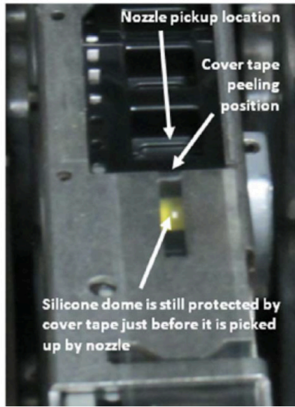
Figure 18. Example of a modified feeder which protects the silicone dome prior to pickup
