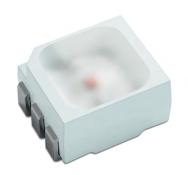
LUXEON 3258 is the perfect RGB package for indoor, architectural, and decorative applications. Its very compact, low profile package – only 1.75mm – can manage up to 0.5W of power and has an IPX8 water resistant rating. Each of the three color channels can be individually addressed and controlled. It pairs perfectly with LUXEON 2835 Architectural white LEDs for additional color changing options.
